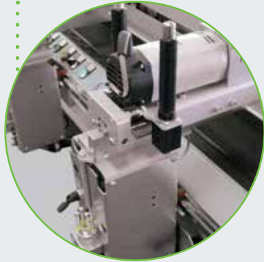
FE-320 Milling unit*... mobile, incl. pneumatic height adjustment with fourfold turret stop top and bottom, collet diameter: 8 mm manual adjustment, two-hand operation and stop for lock case milling (adjustable from 20 to 200 mm) cutter diameter: 12 mm.
