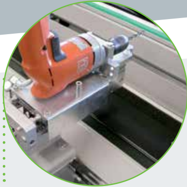
EB-320 Corner bracket drilling unit*... mobile, with quick-change drill chuck, swivel device 0.8°, pneumatic height adjustment with fourfold turret stop at top and bottom, left and right hand stops for the drilling position, with outer scanning and vertical clamping unit.
