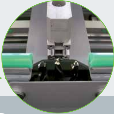
GOB-320 Handle drilling unit*... stationary installation with hydro-pneumatic drill advance clamping unit, three-spindle drilling head 43 mm, inside diameter of sash: approx. 250 mm, drill speed: approx. 550 rpm, drill diameter 12-14-12
