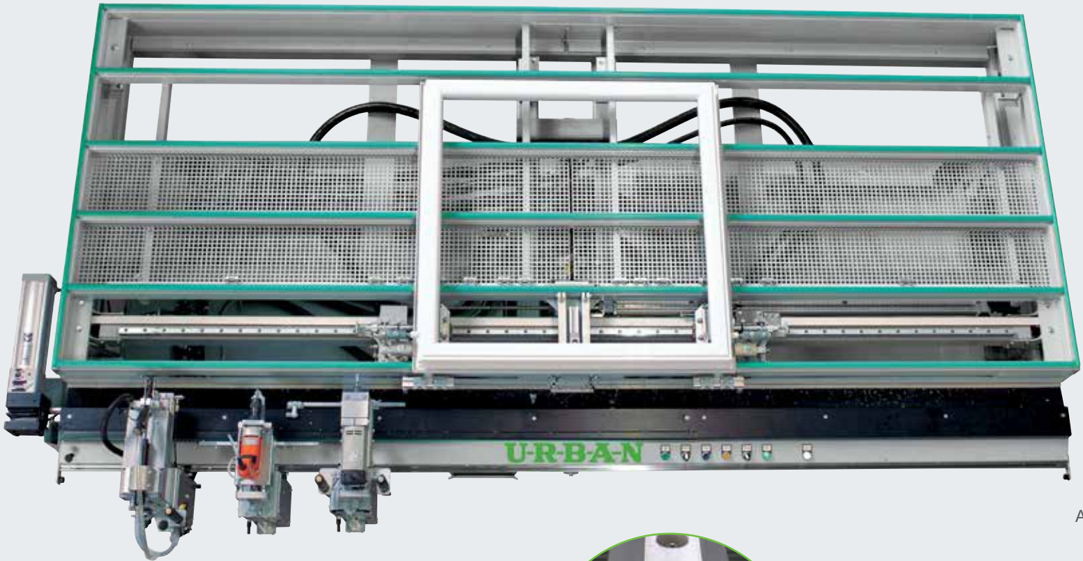
EB-320 Corner bracket drilling unit*... mobile, with quick-change drill chuck, swivel device 0.8°, pneumatic height adjustment with fourfold turret stop at top and bottom, left and right hand stops for the drilling position, with outer scanning and vertical clamping unit.
