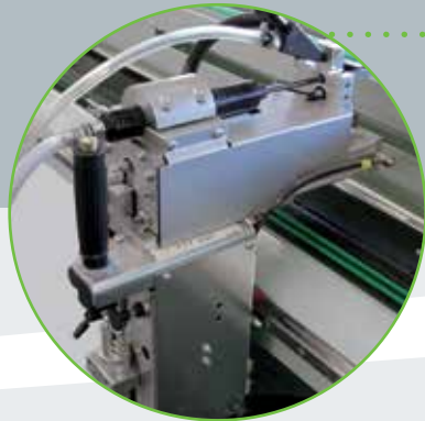
S-320 Screwing unit*... mobile with automatic screwing cycle and fourfold depth switch-off, incl. pneumatic height adjustment and funnel for manual infeed for two screw lengths (possible screw lengths: 20-35 mm), automatic feeding device with switch-off in case of non-use.
