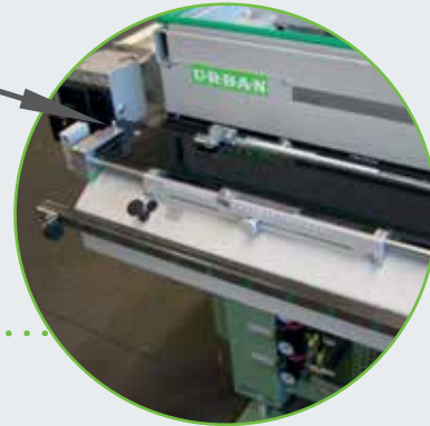
ASKM-320 Stop system*... for centered handle position, automatic function like ASK-320, only possible in combination with ASK-320.
