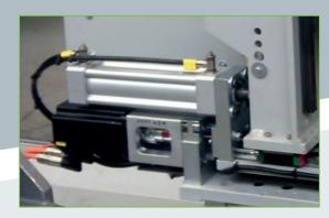
All critical movements controlled by servo drive. Resulting in adjustable table movement parameters. Some of which are: welding pressure, burn off, table synchronization, Joining pressure & final pinch.
