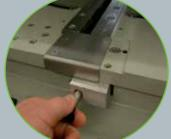
Universal application possibilities... The manually adjustable weld seam limitation from 0.2 mm to 2.0 mm allows best results when welding white and laminated profiles.
