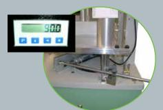
Highest precision... Due to the direct measuring at the stop rail the digital angle indication guarantees absolute precision.
